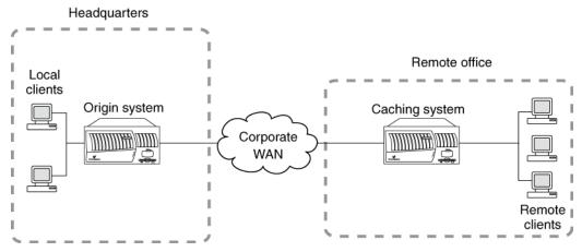
Figure 5: Typical FlexCache WAN Deployment
