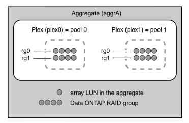
Figure 4: Aggregate with two (mirrored) plexes using array LUNs
