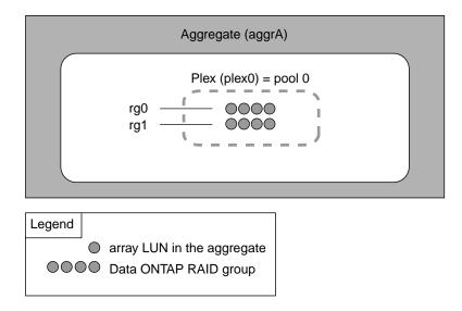
Figure 2: Unmirrored aggregate with array LUNs
